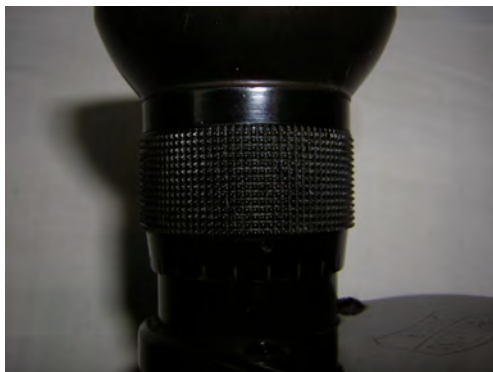
illustr. 3 horizontal/vertikal knurling
