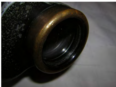
illustr. 9 - round housing without grooves (ex.:CARL ZEISS JENA - DF 8X (= Telact), # 498514 )
