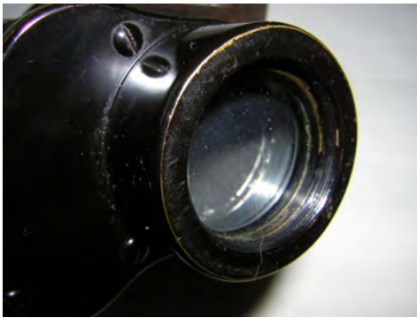
illustr. 1 solid union of bottom plate and objective housing ( ex: DF 6 X ( 21) # 135.772 )
