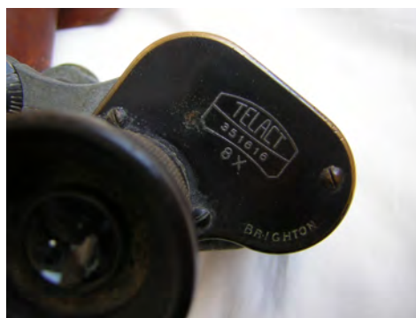
illustr.11 - 3 screws on top plate - ( - Carl Zeiss London – TELACT 351.616 -)
