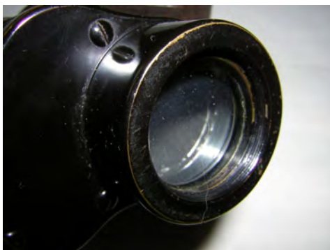
illustr. 1 solid union of bottom plate and objective housing ( ex: DF 6 X ( 21) # 135.772 )
